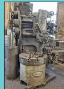
26" Swing/30 HP Bullard Vertical Turret Lathe
