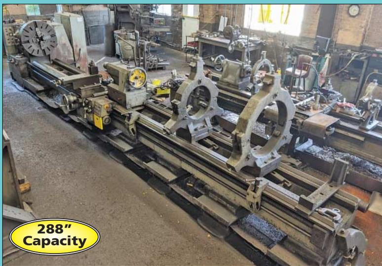
20" / 26" X 288" Poreba TPK 80/90A Gap Bed Lathe
