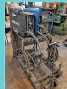
Miller XMT-350 CC/CV Weld Power Source with Miller Suitcase X-Treme 12 VS Wire Feed
