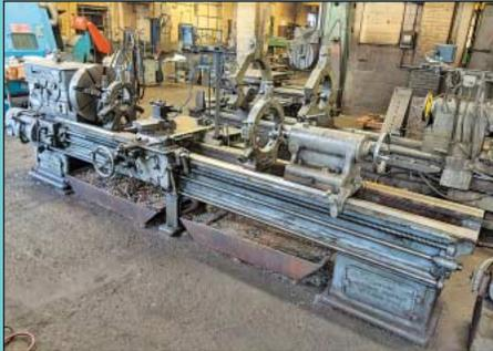
14" X 152" Lehman "Hydrotral" Engine Lathe
