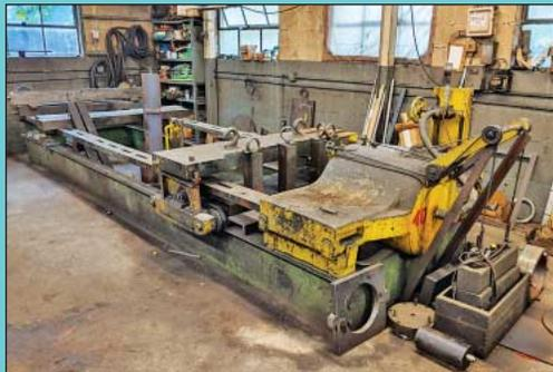
300 Ton (Est.) Floor Type Horizontal Hydraulic Press
