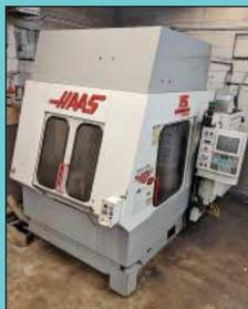
Haas Model HS-1 CNC Horizontal Machining Center
